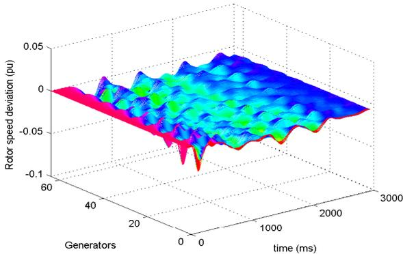
Fig. 7. Rotor speed deviation of all machines with applying conventional PSS.
