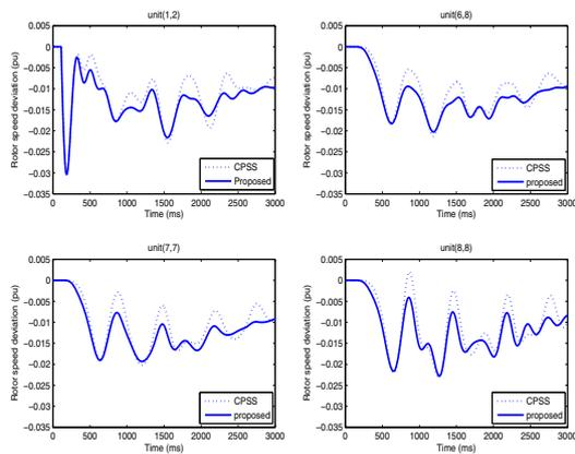
Fig. 11. Rotor speed deviation for selected machines before and after applying the proposed modifications of PSS.
