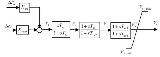
Fig. 2. Block diagram of a conventional PSS.
