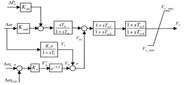
Fig. 3. Block diagram of the proposed modification of PSS.
