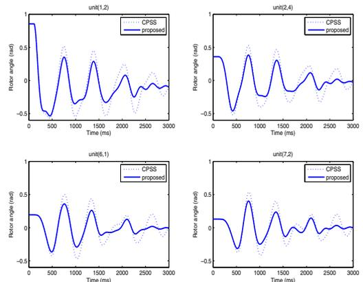
Fig. 10. Rotor angle for selected machines before and after applying the proposed modifications of PSS.
