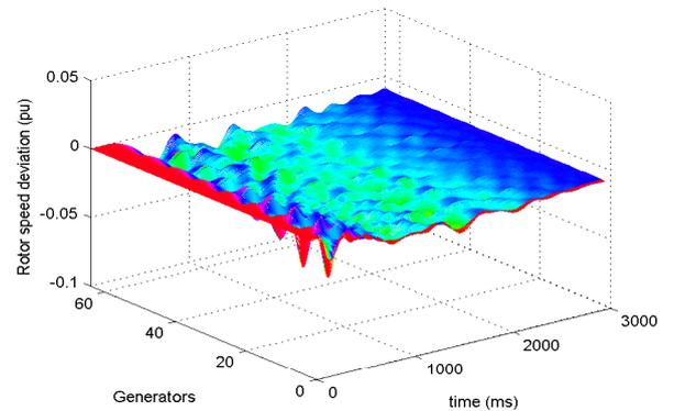
Fig. 9. Rotor speed deviation of all machines with applying the proposed modifications of conventional PSS.
