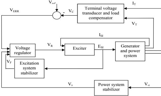
Fig. 1. Block diagram of general functional of excitation control system.
