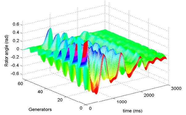
Fig. 8. Rotor angle of all machines (referred to machine(8,8)) with applying the proposed modifications of conventional PSS.
