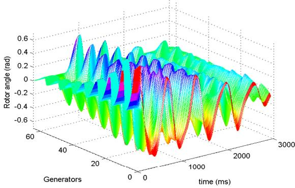
Fig. 6. Rotor angle response for all machine (referred to machine(8,8)) with applying the conventional PSS.
