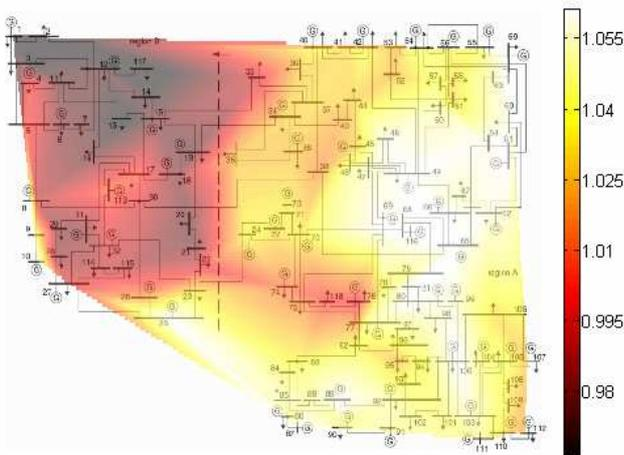
Figure 8: Interpolated voltage level across the IEEE 118 Bus System by Case #3. Voltage is in p.u.
