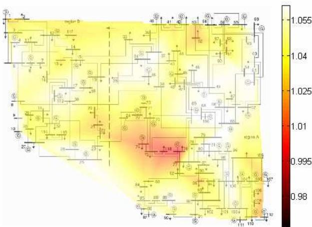
Figure 9: Interpolated voltage level across the IEEE 118 Bus System by Case #4. Voltage is in p.u.
