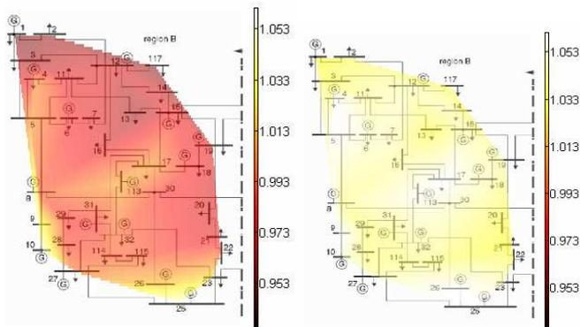
Figure 5: interpolated voltage level across the Region B of the IEEE 118 Bus System. On the left, reactive power reserves are maximized. On the right, active power losses are minimized. Voltage is in p.u.
