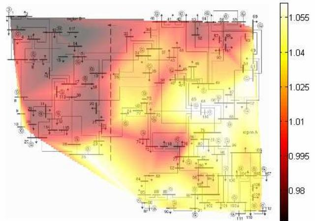
Figure 6: Interpolated voltage level across the IEEE 118 Bus System by Case #1. Voltage is in p.u.
