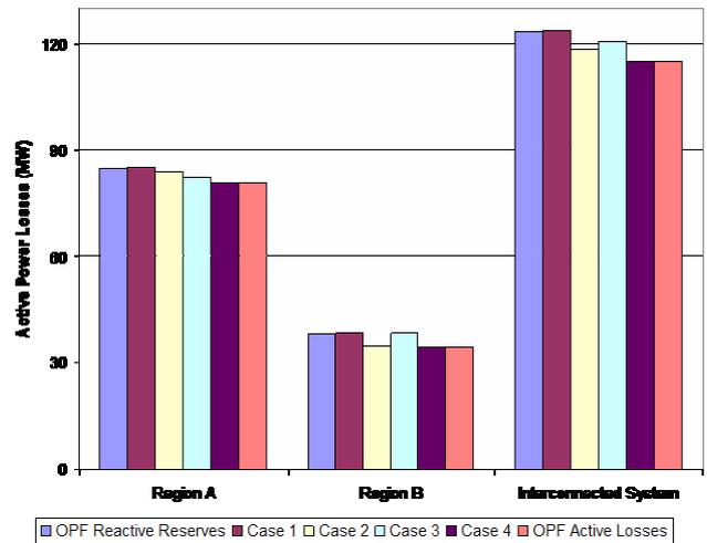
Figure 10: Active power losses in Region A, Region B and in the interconnected power system
