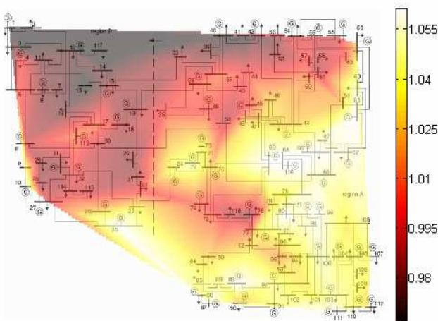
Figure 2: Interpolated voltage level across the IEEE 118 Bus System where the global amount of reactive power reserves has been maximized. Voltage is in p.u.
