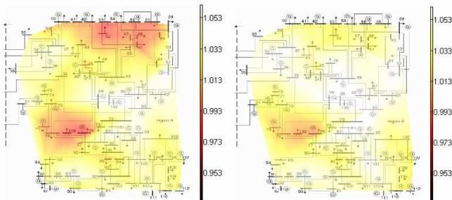
Figure 4: Interpolated voltage level across the Region A of the IEEE 118 Bus System. On the left, reactive power reserves are maximized. On the right, active power losses are minimized. Voltage is in p.u.
