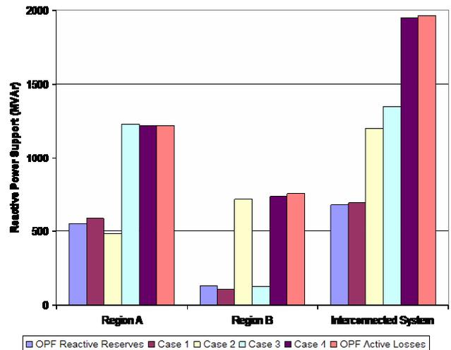
Figure 11: Reactive power support in Region A, Region B and in the interconnected power system
