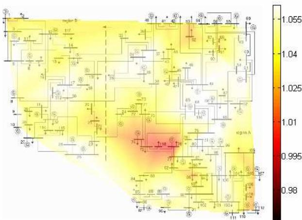
Figure 3: Interpolated voltage level across the IEEE 118 Bus System where the global amount of active power losses has been minimized. Voltage is in p.u.
