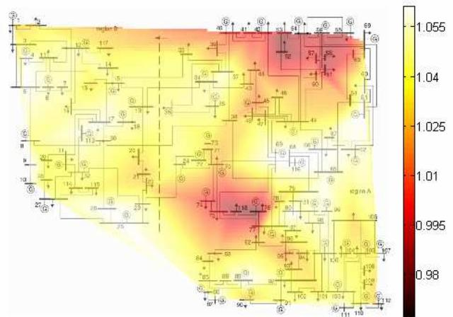
Figure 7: Interpolated voltage level across the IEEE 118 Bus System by Case #2. Voltage is in p.u.
