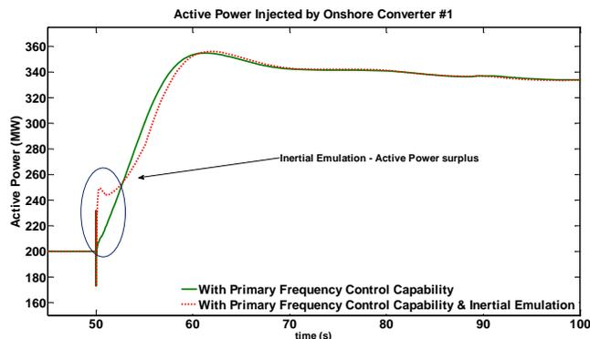
Fig. 11. Active power injected on AC network Area#1 with and without inertial emulation capability.
