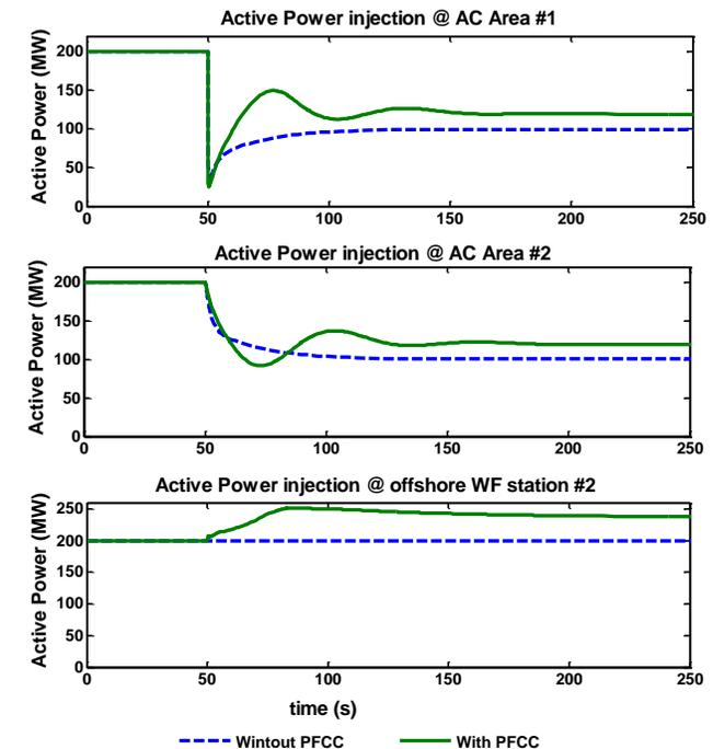
Fig. 13. Active Power at AC Area#1, AC Area#2 and offshore WF#2 HVDC-VSC converter.
