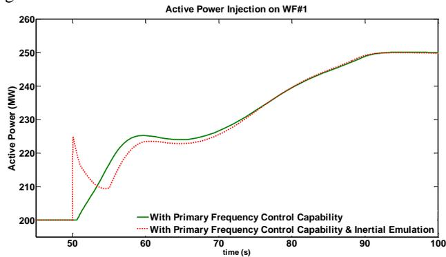
Fig. 10. Active power injected by WF#1 with and without inertial emulation capability.
