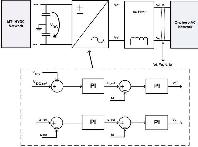
Fig. 2. Internal control loops of the onshore converters.
