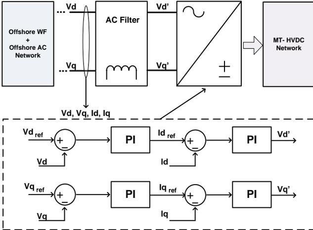
Fig. 3. Internal control loops of the offshore converters.
