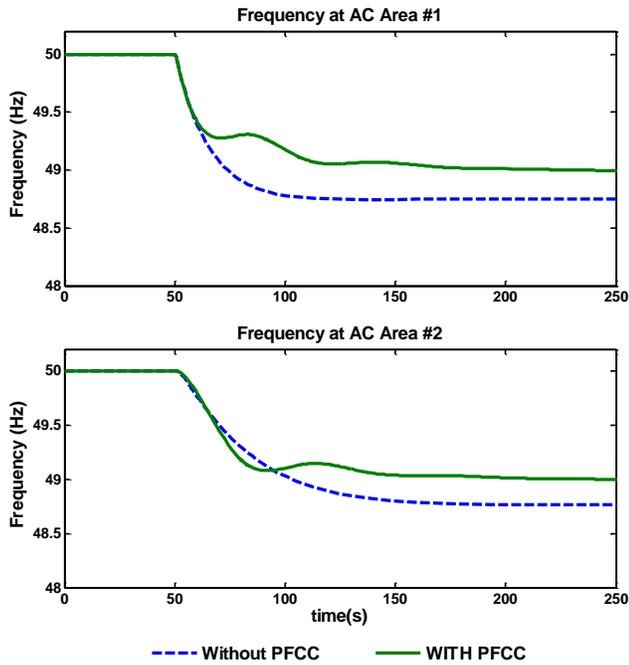
Fig. 14. Frequency behavior at AC Area#1 and AC Area 2.
