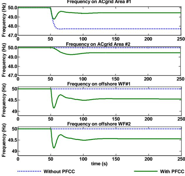
Fig. 7. Frequency behavior in AC-sides.
