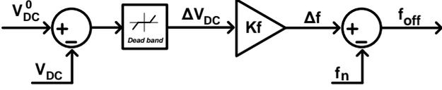
Fig. 5. Droop control mechanisms for HVDC-VSC offshore AC grid frequency.
