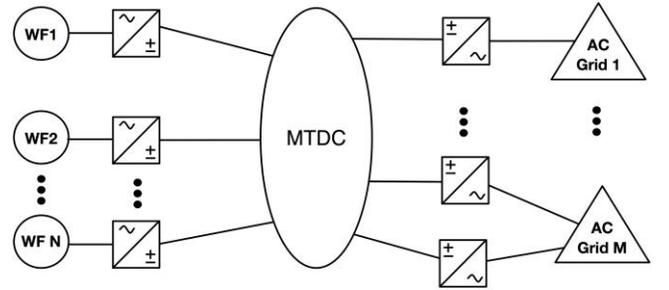
Fig. 1. Conceptual architecture of a MTDC grid.
