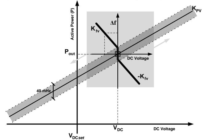
Fig. 4. Droop control mechanisms for HVDC-VSC onshore converter stations.
