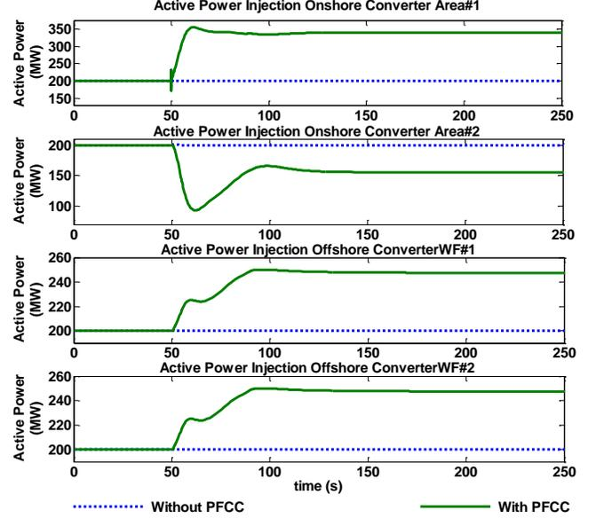
Fig. 9. Active power injection at each MTDC network terminal.
